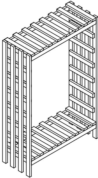
2. Nail only the bottom shelf to the side rail. Leave the top shelf to keep the spacing.
